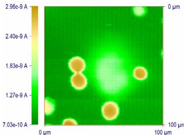
**Figure 2.** SECM image of a polycarbonate filtration membrane with a 2- $\mu$ m-diameter Pt disk UME in  $Fe(CN)_6^{4-}$  solution. Average pore diameter is ca. 10  $\mu$ m. the oxidation of ferrocene at a Pt UME has been
