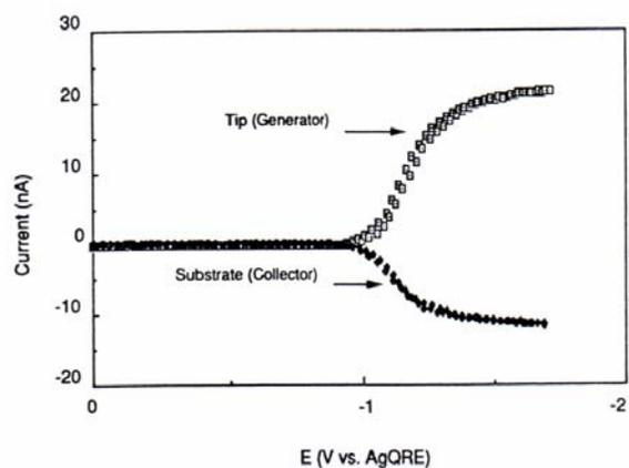
**Figure 4.** SECM voltammograms for FN (28.2 mM) reduction in TG/SC mode.  $d = 1.8$   $\mu\text{m}$ .  $E_T$  was scanned at 100 mV/sec with  $E_S = 0.0$  V vs AgQRE. (Reprinted with permission from Ref. 5a, copyright 1992, American Chemical Society.)
