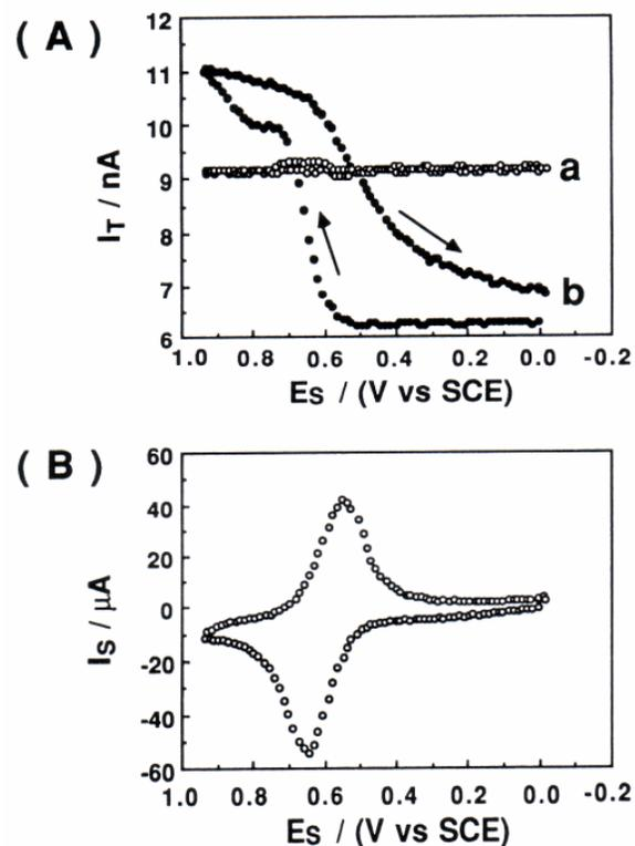
**Figure 6.** T/S CVs (A) curve a,  $d = 500 \mu\text{m}$ , and substrate CV (B) on Nafion/ $\text{Os}(\text{bpy})_3^{3+/2+}$  electrode in  $\text{K}_3\text{Fe}(\text{CN})_6/\text{Na}_2\text{SO}_4$ , scan rate =  $50 \text{ mV/sec}$ ,  $E_T = -0.4 \text{ V vs SCE}$ . (Reprinted with permission from Ref. 6a, copyright 1990, American Chemical Society.)
